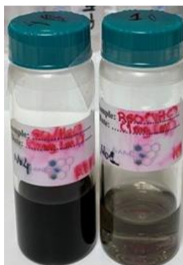
Figure 12: Digital picture of GO & rGO dispersions.
