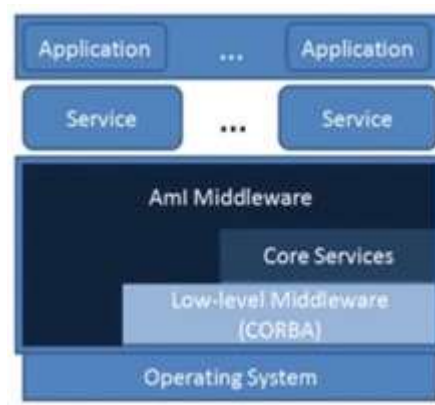
Figure 12: The structure of Aml Middleware
