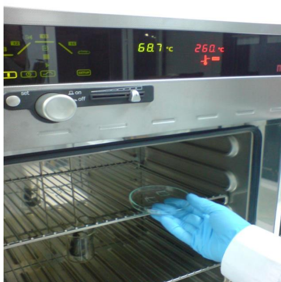
Fig. 5.7 Placement of the substrates in oven.
