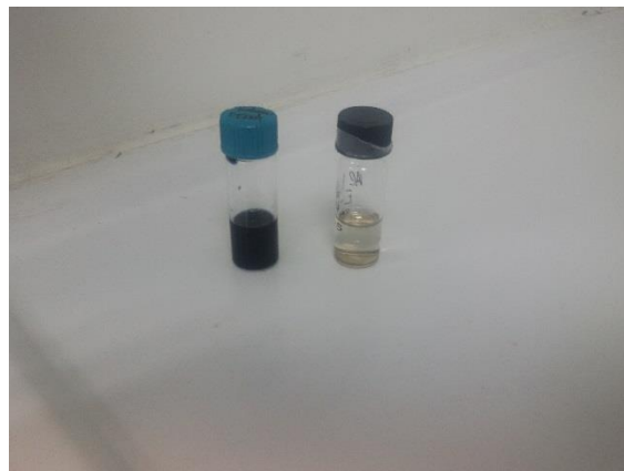
Fig. 5.3 PEDOT:PSS (left) and Al NPs in Ethanol (right).
