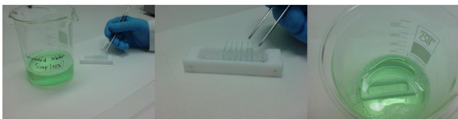
Fig. 5.5 Preparation for substrate cleaning.
