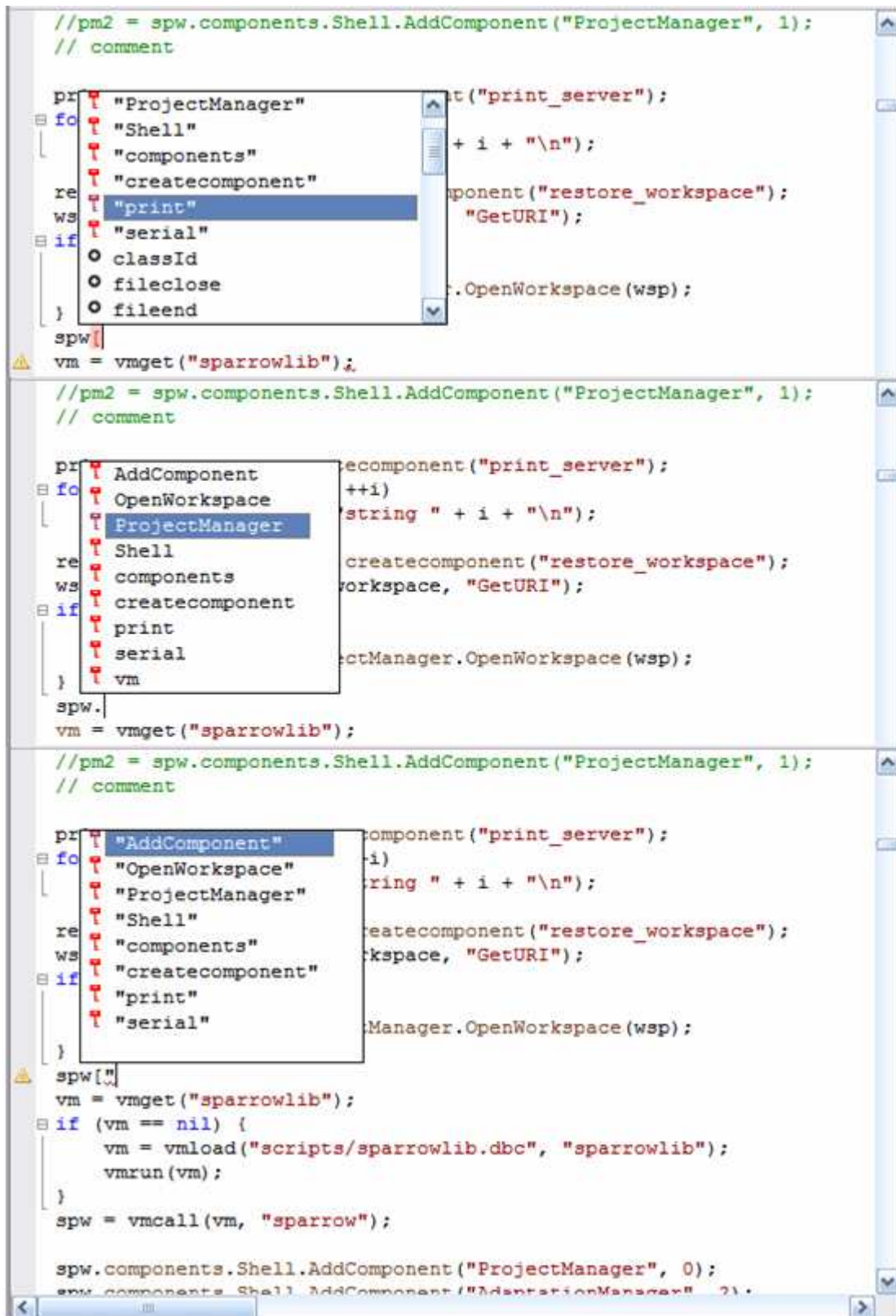
Figure 28 - Automatic completion of symbols, and object members as ids and strings
