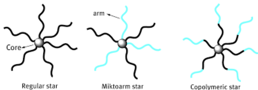
Figure 3 - Representation of structure in star polymers [8]
