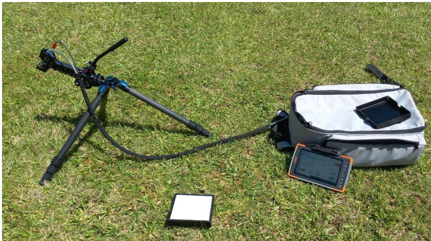
Figure 2) The radiometer and the spectral diffuse panel
