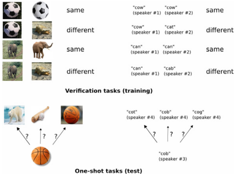
Figure 2.6: Siamese Nets: Training and testing procedure. Taken from [14].
