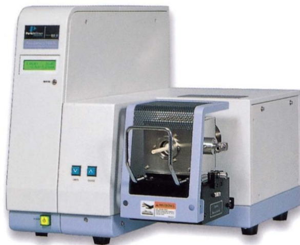
Figure 2.4: Perkin Elmer Pyris Diamond TG/DTA.
