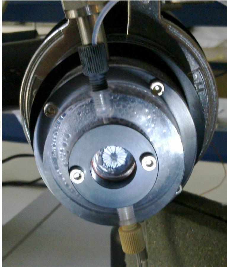
**Figure 12.** View of the Impactor plate with the asterisk-like pattern.
