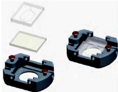
Figure 3.2: Illustration of resealable chip interface and microfluidic devices [45] .
