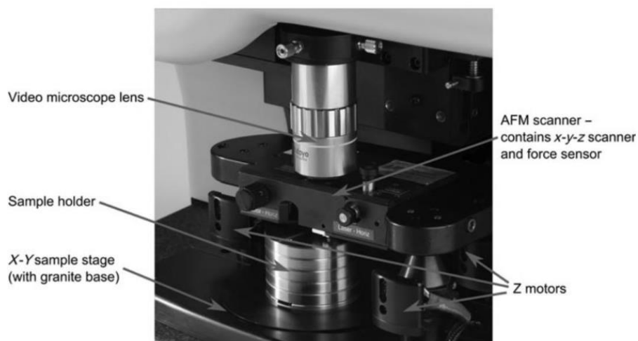
Figure 42 AFM stage and its components
