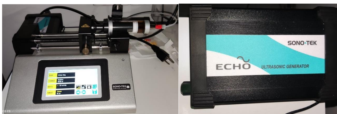
Figure 16 High accuracy pump syringe, ultrasonic generator
