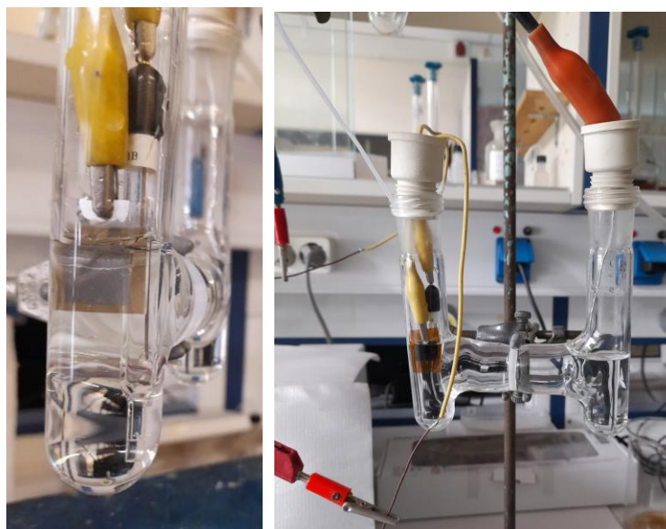
Figure 44 Electrocatalysis for H 2 production setup
