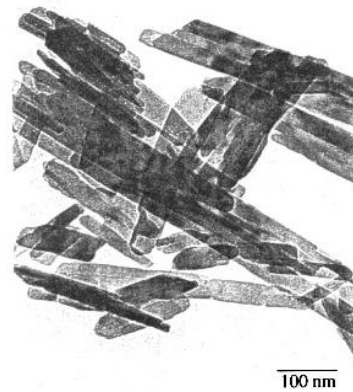
Figure 4. Transmission electron microscopy pictures of HAP crystals. (Koutsopoulos 2002)
