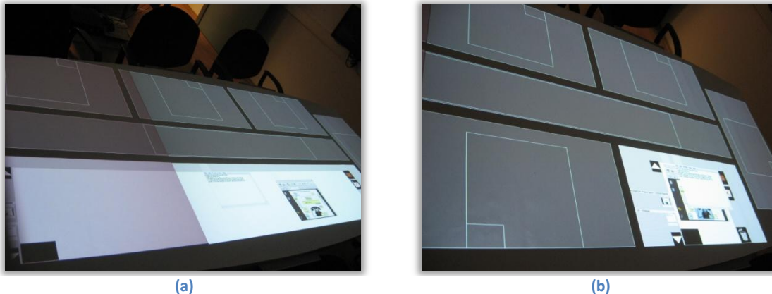
Figure 41. Dynamic area shrinking. The user initially occupies three working areas (a), then shrinks the personal working area to the rightmost area (b)
