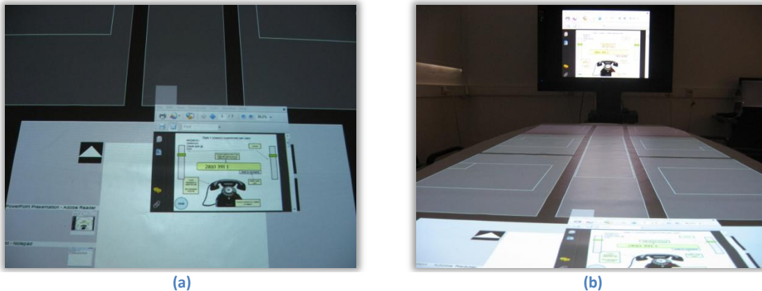
Figure 44. Public display of documents. The user drops a document's handle within the public area (a), a large copy of that document automatically appears on the secondary display (b)
