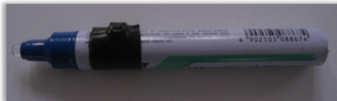
Figure 50. A custom IR pen used on the SMURF Table
