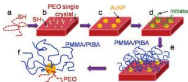
Figure 30. Schematic illustration of the preparation of polymer-functionalized Janus Au-NPs by combining solid-state "grafting-to" and "Grafting-from" methods.
