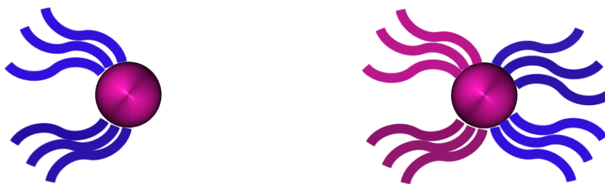
Figure 27. Types of hybrid Janus nanoparticles; (left) one side of the particle is covered by polymer chains; (right) the particle's core covered by a compartmentalized shell.
