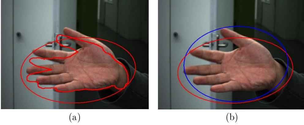
Figure 3.5: In (a) the Gaussian kernel of position \vec{\theta}_{t-1} and covariance \Sigma_{t-1} , as well as the prior object shape mask M_{t-1} from previous I_{t-1} are illustrated, both superimposed on image frame I_t and colorized in red. Image in (b) illustrates the previous Gaussian kernel in red and the newly estimated Gaussian kernel in blue. The latter is computed by the tracking method for I_t , providing an updated position \vec{\theta}_t and covariance \Sigma_t of the tracked object.
