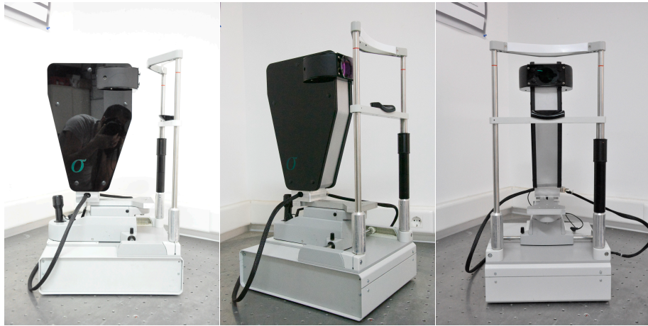
Figure 68 The developed compact system for optical measurements of forward scattering
