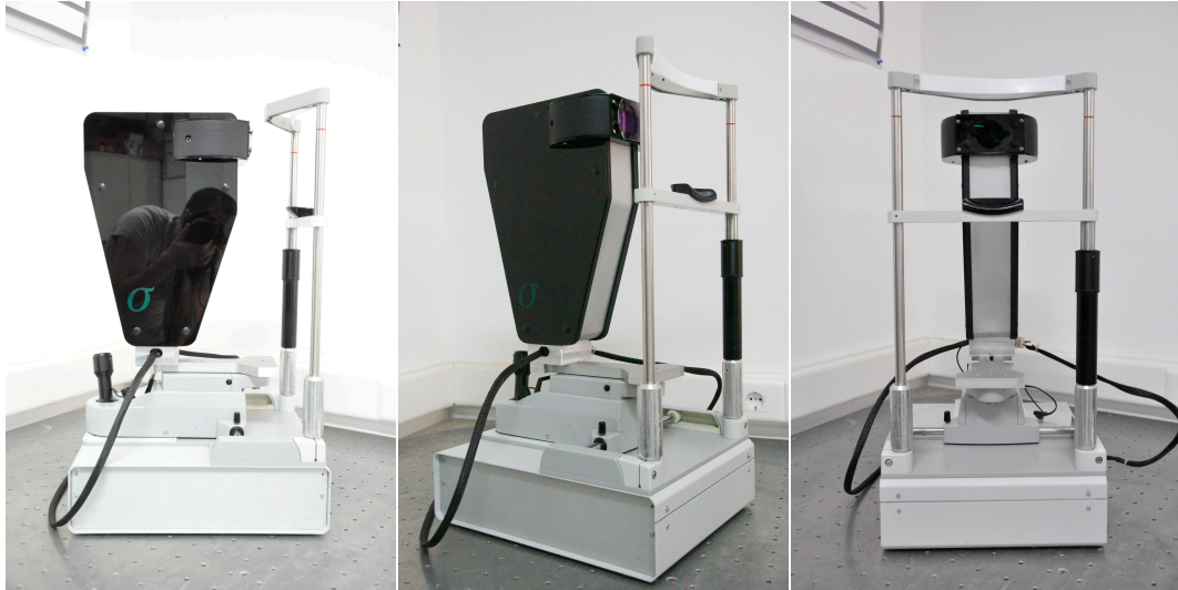
Figure 44 The developed compact system for optical measurements of forward scattering
