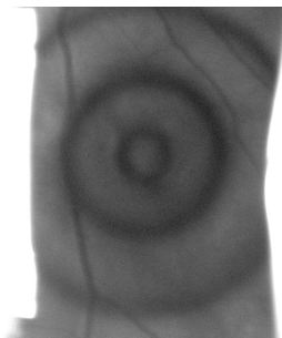
Figure 30 Actual image of the projected LED source on the fundus.
