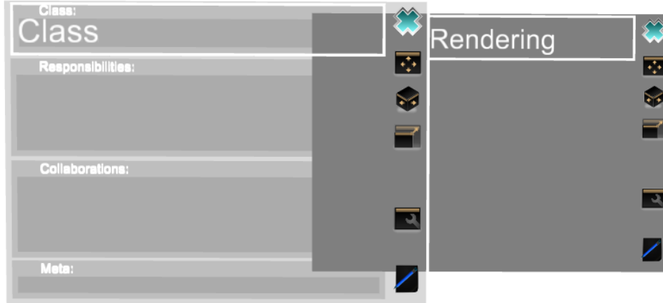
Figure 5.3: Current transparency rendering. Controls are not blended with the transparent window (Class is the transparent card).
