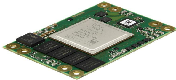
Figure 2.1: The Trenz TE0808 system-on-module (SoM), featuring a Zynq Ultrascale+ FPGA
