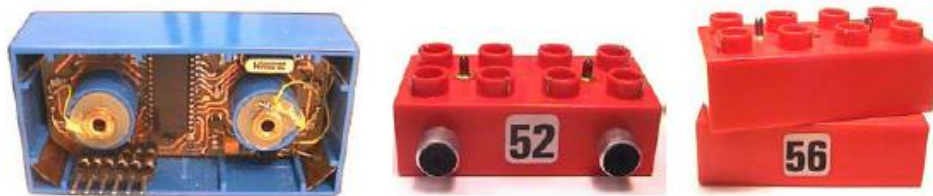
Figure 5. I-BLOCKS, augmented building blocks for programming through a tangible user interface. © H. H. Lund, 2002.
