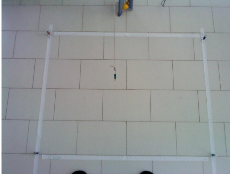
Figure 14. Wii Remote recognition scope at 3 m height.
