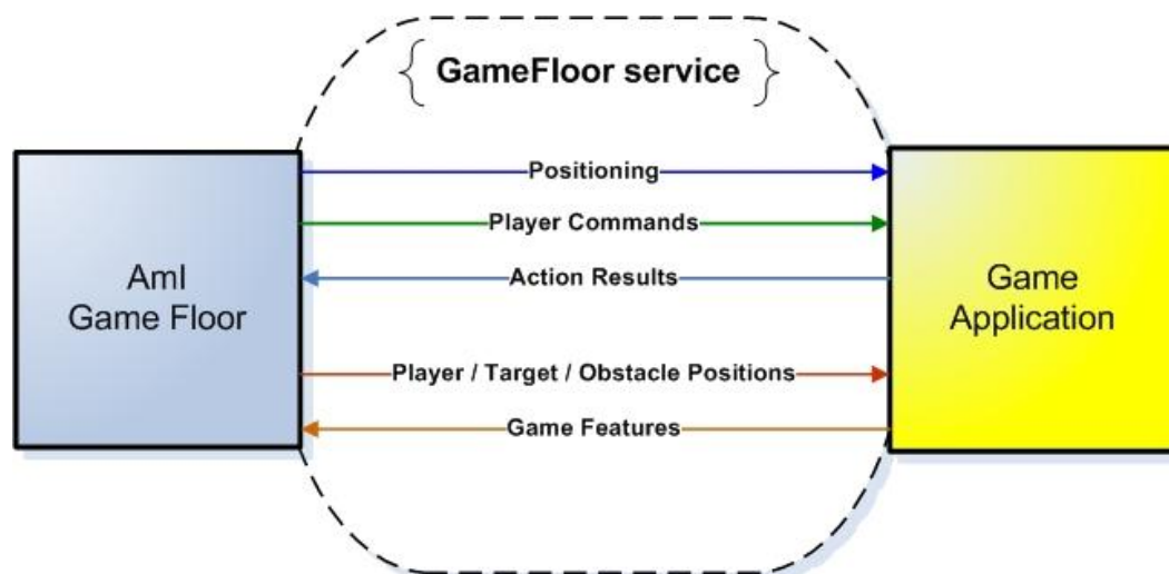
Figure 33. Typical Data exchange between Aml Game Floor and applications
