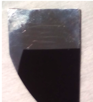
Figure 6.12: Sample IV: 1.75 \mu\text{m} Aluminum step on Si substrate.
