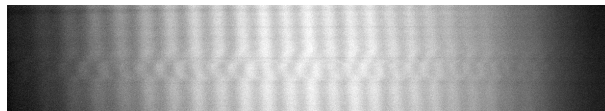
Figure 6.6: Spectral fringes from the 9.5 \mu\text{m} nominal value of Stylus profilometer's groove depth.
