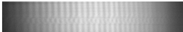
Figure 6.5: Spectral fringes from the 9.3 \mu\text{m} nominal value of Stylus profilometer's groove depth.
