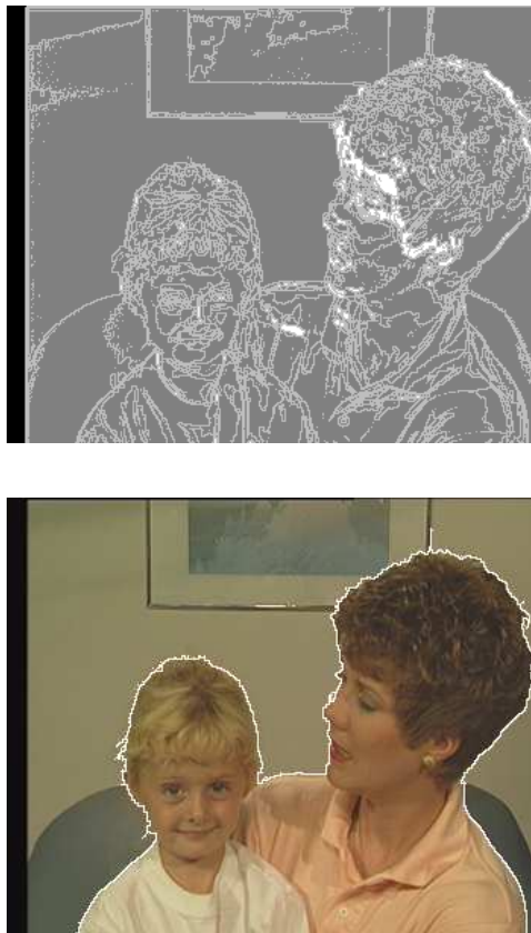
Figure 6.11: Initialization (up) and moving objects extraction result (down) for frame 42 of the sequence “ Mother ”.
