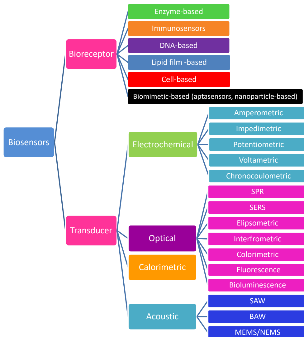
Figure 3. Classification of biosensors, bioreceptors and transducers. LSPR-Localized Surface Plasmon Resonance; SPR – Surface Plasmon Resonance; SERS - Surface-enhanced Raman scattering; SAW – Surface Acoustic Wave; BAW – Bulk Acoustic Wave; MEMS/NEMS - micro/nano-electromechanical.
