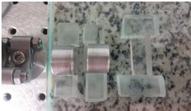
Figure 6.7 Glass breadboard made of soda lime glass.
