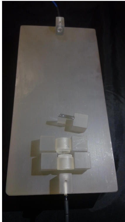
Figure 7.19 Assembled Zerodur breadboard. Visible are the pair of wedges with their holding blocks, a glass plate with a holding block and two zerodur fiber couplers facing each other.
