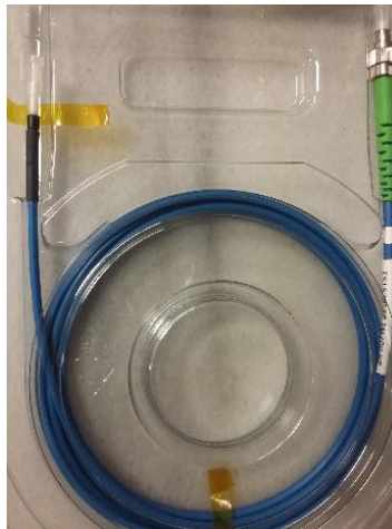
Figure 7.6 Thorlabs PM780-HP fiber with FC/APC connector on right side and bare ceramic ferrule on left side.
