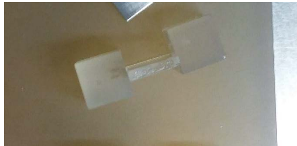
Figure 7.18 Zerodur blocks holding in position the glass plate.
