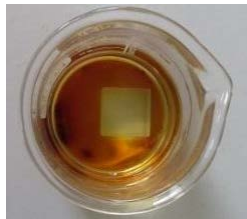
Figure 4.10 Zerodur block inside a bath of chromic acid.
