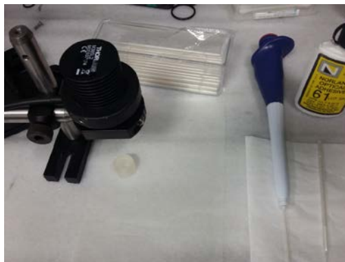
Figure 7.10 Wedge holder just before applying the adhesive.
