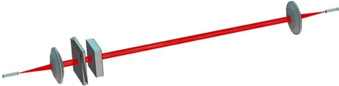
Figure 1.2 Breadboard with corrective optics. A pair of wedges aligns the beam while the plate displaces it.
