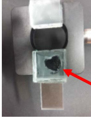
Figure 7.15 The glass plated attached to the glass block. A drop of Loctite401 in the middle of the glass block is also clearly visible.
