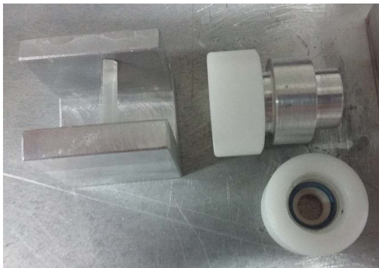
Figure 6.2 Wedge mount and aluminum holders for the glass plate.
