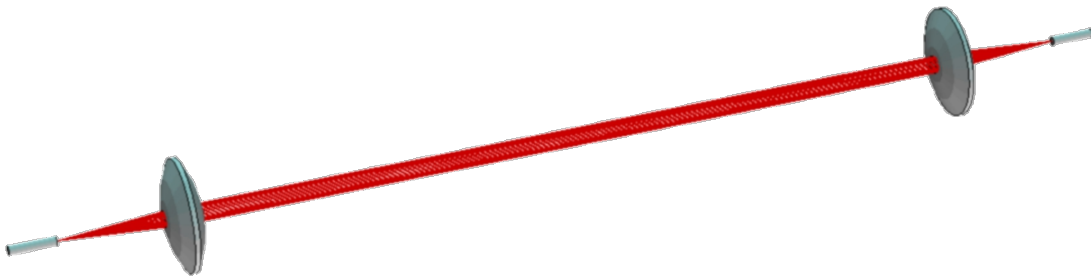
Figure 1.1 Simple breadboard consisting of a transmitting fiber-lens and receiving fiber-lens.
