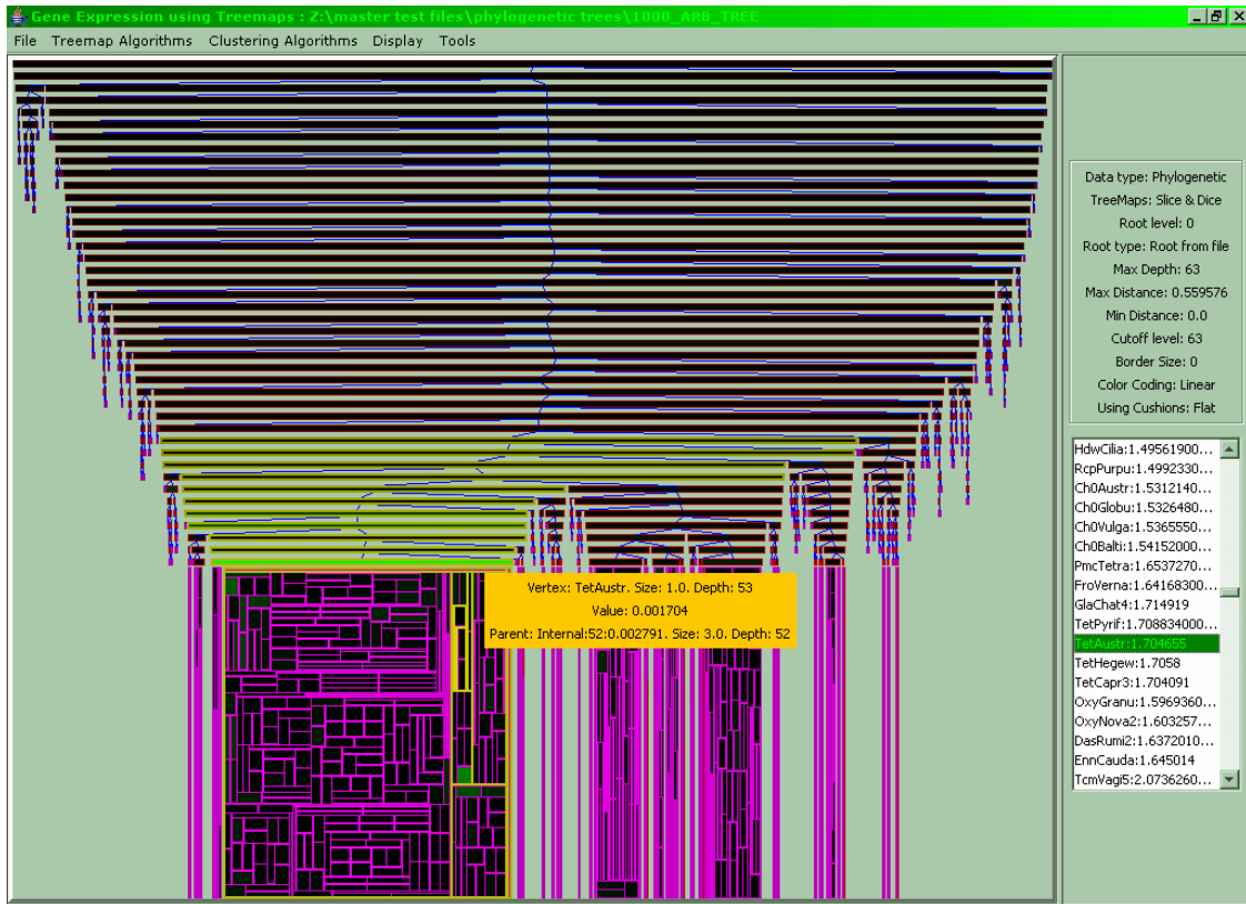
Figure 6.5.3.2: Whenever the user selects a node from the list on the right the corresponding node is located, selected and information about it displayed
