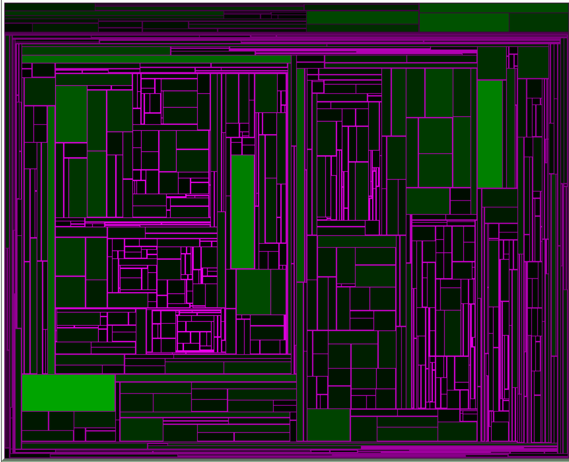
Figure 6.3.3.3: A treemap with 1000 leaves and all leaves sizes set to their normalized weight, the brightest nodes are also the biggest
