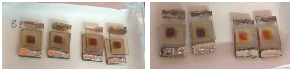
Figure 4.24 Pictures of the fabricated DSSCs.
