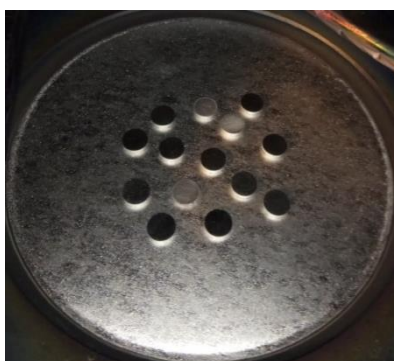
Fig. 6.26: Niobium pellets on the nickel target
