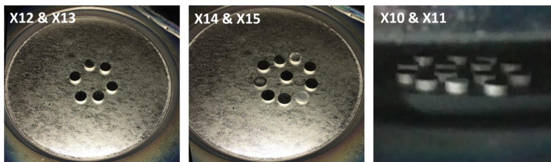
Fig. 6.10: Niobium pellets on the nickel target of sputtering chamber
