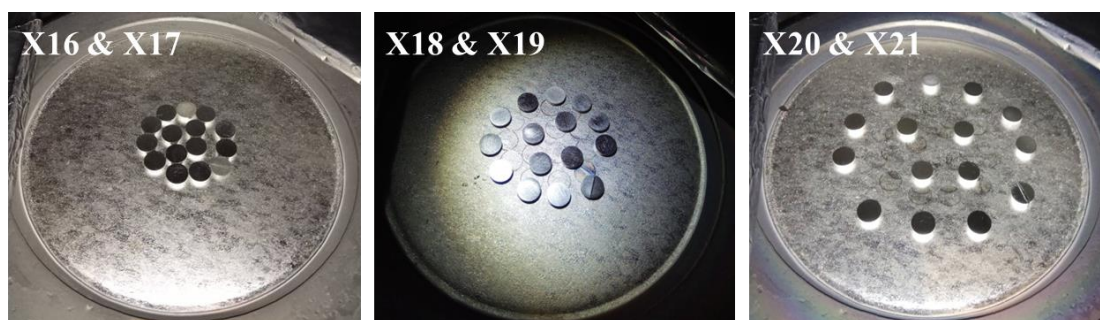
Fig. 6.18: Niobium pellets on the nickel target of sputtering chamber
