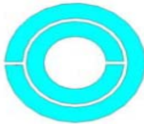
Σχ. 1.5: Split Ring Resonator (SRR)
