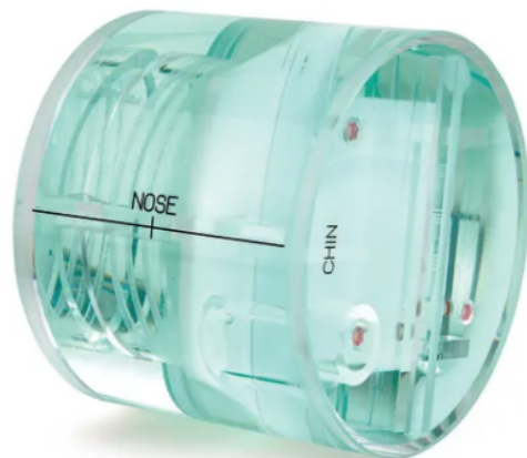
Figure 1.1: The ACR MRI Phantom, which is employed in clinical practice to ensure the quality of MRI scanners for quality assurance purposes.
