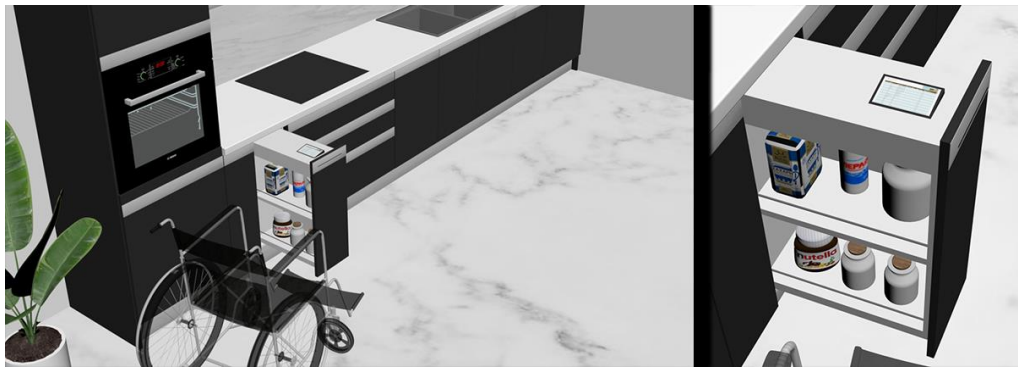
Figure 9 : 3D representation of the accessible smart kitchen cupboard placed in a typical kitchen.
