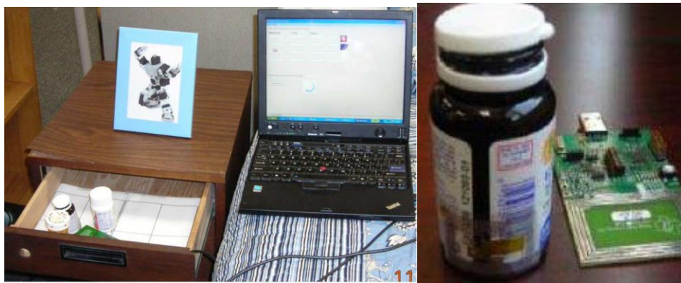
Figure 7 : Smart Drawer [21]: Left: Smart Drawer system, Right: RFID reader and RFID tags on a bottle
