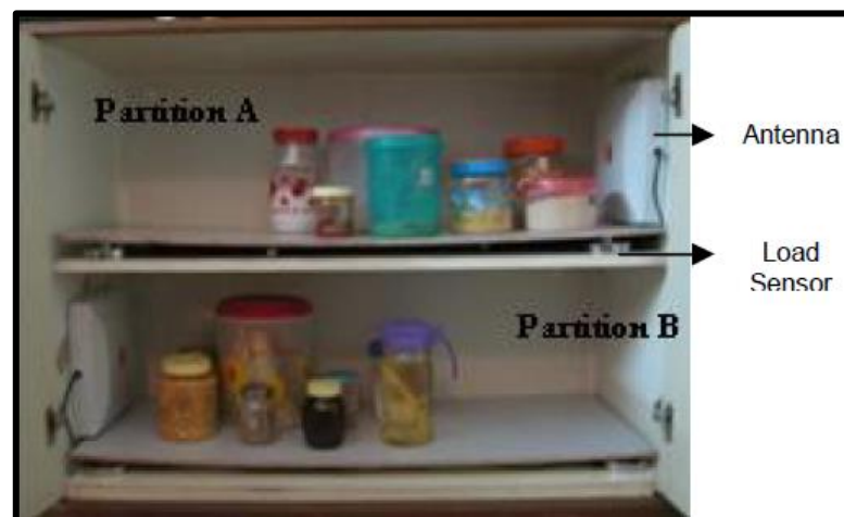
Figure 3 : Smart kitchen Cabinet [16], System equipped with RFID readers and load sensors.
