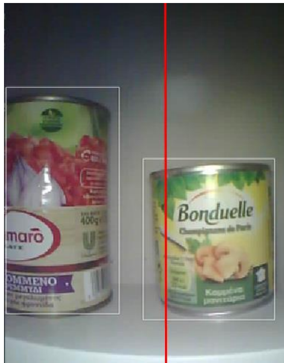
Figure 22 : The camera detected a tomato can (Left) and a mushroom can (Right). The lazer detector line (Red) is included only in the mushroom's white rectangle that's why the image of the right product will be the only one that would be cropped and saved locally. As the camera moves, the red line will keep scanning to the left the rest of the stored products.
