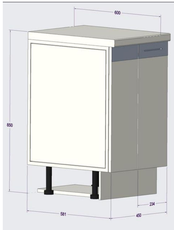
Figure 10 : Dimensions of the Accessible Smart Kitchen Cupboard prototype
