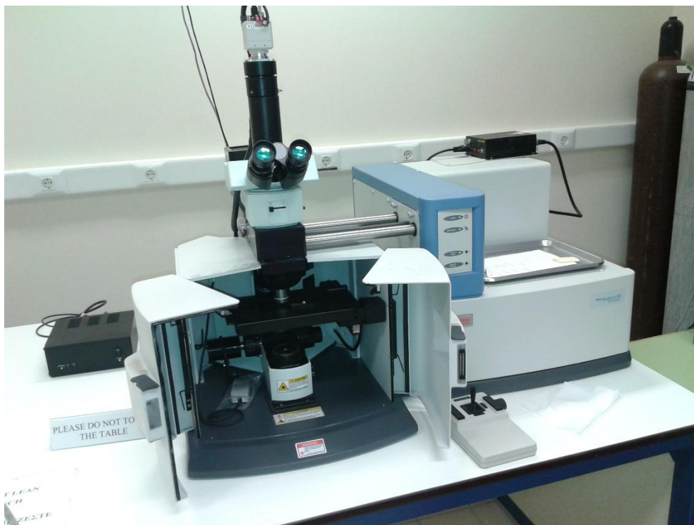
Figure 3.1: Nicolet Almega XR Micro Raman analysis system.
