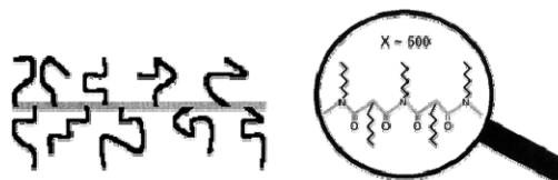
Figure III-1: Diblock copolymer nanofiber consists of a crosslinked cylindrical core made of one block and surface-anchored chains made of another block.
