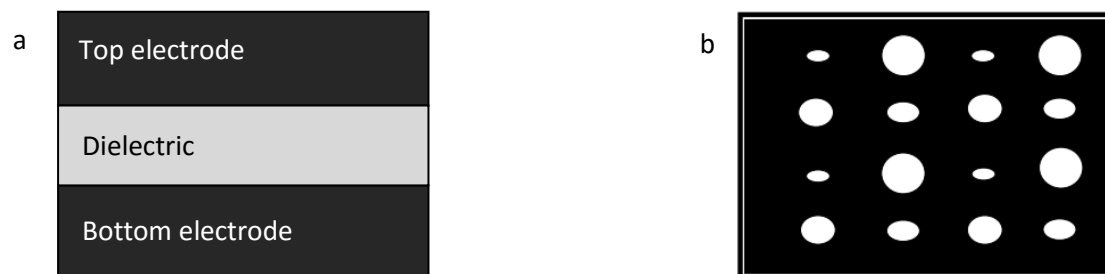
Fig.38: Schematic illustration of the MIM test devices. a) the typical structure of a MIM capacitor, b) the final form of the test device, with different size MIM capacitors. One period of each sample consists of four different in size capacitors. The top electrode of each different capacitor has a diameter of 226\mu\text{m} , 176\mu\text{m} , 126\mu\text{m} and 46\mu\text{m} respectively.
