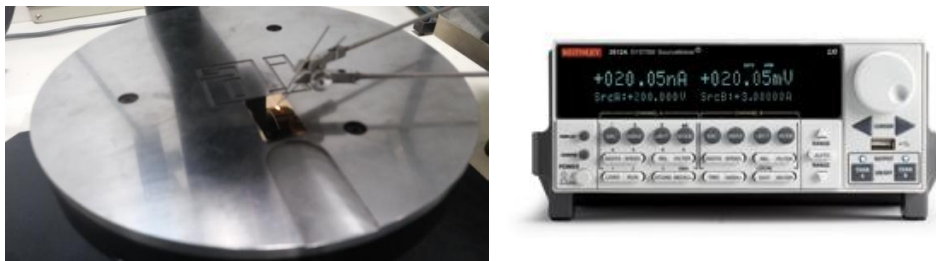
Fig.39: Probe station and semiconductor parameter analyzer (Keithley 2612) which are used for the measurements conduct.
