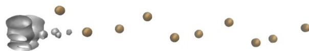
Figure A8: Plane (111) of the Cu-11 atom layer slab (yz plane). the first atom has \sim 87,1\% probability. It is a clear surface state.
