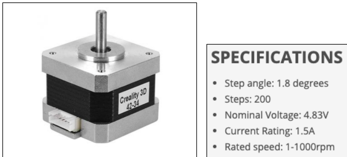
Figure 15: Creality 3D 42-34 stepper motor and datasheet of capabilities presentation. (Figure provided by Grobotronics.gr)
