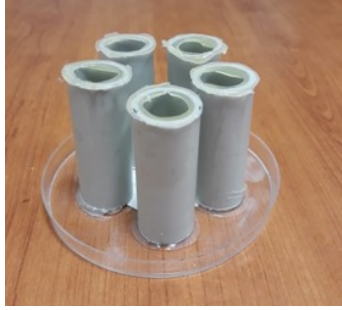
FIG. 14. Experimental configuration of the five-rod unit cell. Five cylinders filled with deionized water, forming a canonical pentagon, were adjusted onto a circular glass base.
