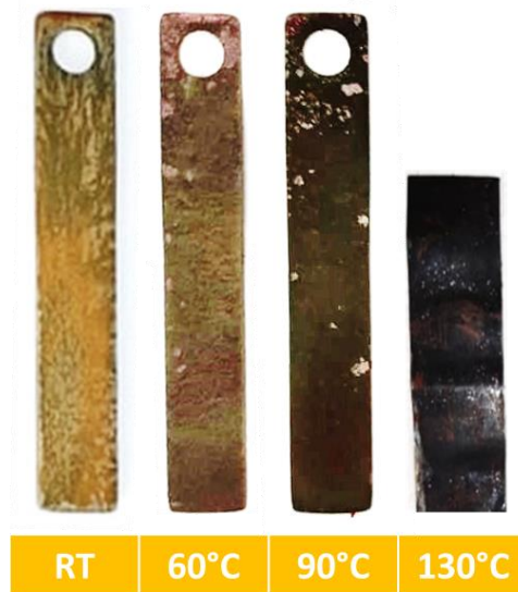
Figure 4.2. Corroded carbon steel surfaces of the specimens exposed to “control” solutions in Brine 2 at pH 7.
