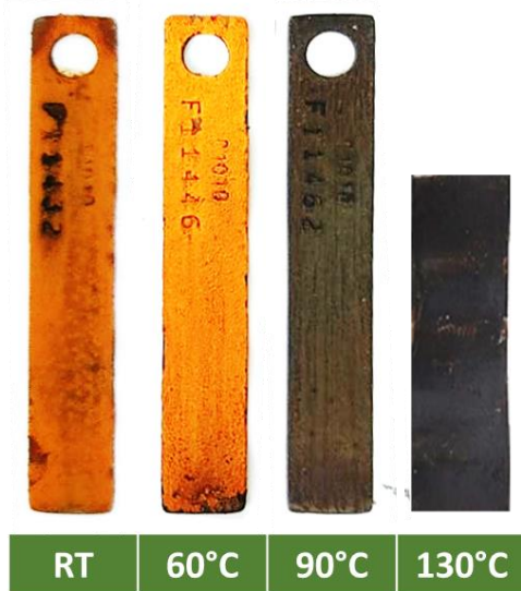
Figure 5.2. left Corroded carbon steel surfaces of the specimens exposed to “control” solutions in deionized water at pH 7.
