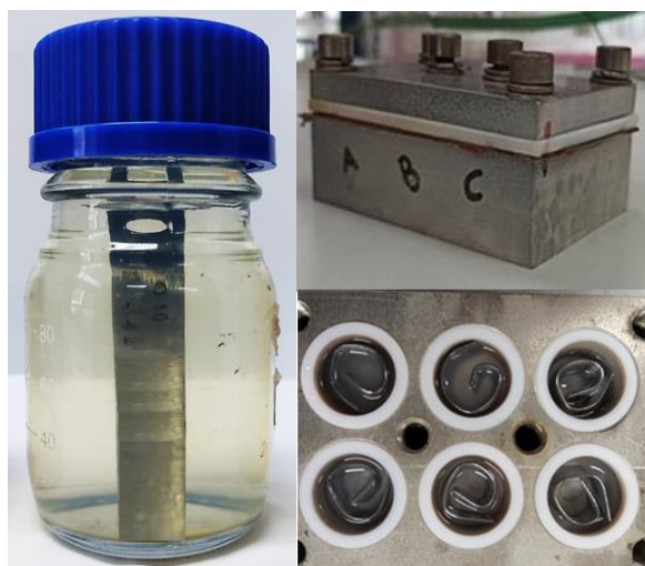
Figure 2.11. Experimental set-up depending on the desired conditions. left Glass bottles with screw caps for corrosion experiments at RT, 60 °C and 90 °C and right High-throughput system containing multiple reaction vessels for HP-HT corrosion experiments (upper: side-view, lower: top view).
