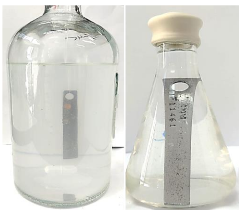
Figure 2.12. Experimental set-up depending on the desired conditions. Left: Glass bottles with screw caps for corrosion experiments at RT under stirring. Right: Erlenmeyer flasks for corrosion experiments in the presence of 50 ppm S^{2-} .
