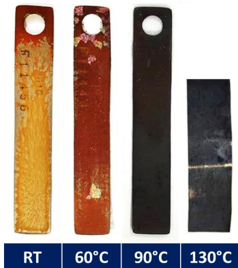
Figure 3.2. Corroded carbon steel surfaces of the specimens exposed to “control” solutions in Brine 1, at pH 7.
