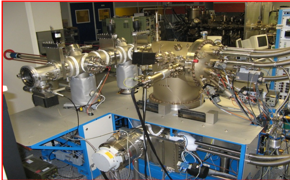
Figure 2.3 Photographic image of the Riber 32P MBE system used for the epitaxy of the InN heterostructures and nanopillars reported in this work. It consists of the conventional Knudsen cells for the supply of In, Ga and Al atomic beams with two additional sources for Be and Si. An Oxford Applied Instruments HD-25 RF plasma source is employed to produce atomic nitrogen species. The equipment is installed in a 100 m 2 clean room of class 1000.
