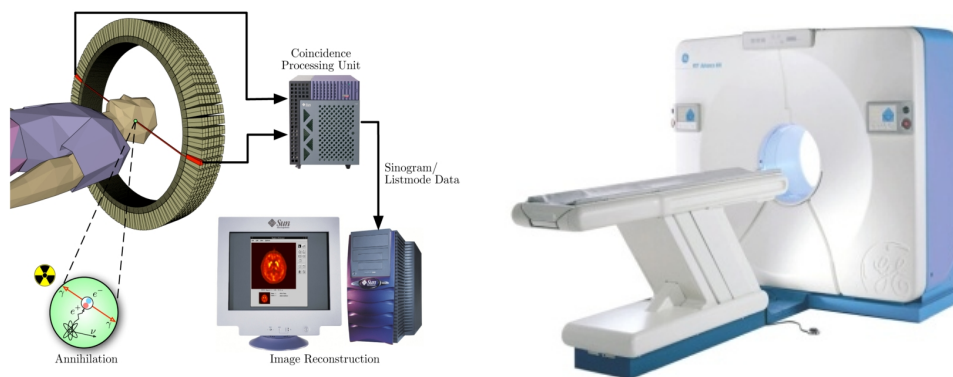
Image I3: (Left) Diagram of a PET device and its basic operational parts (right) image of a PET scanner
