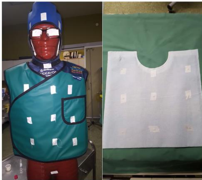
Fig.1 TLDs placed on Rando anthropomorphic phantom and on drape
