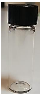
Figure 2.2: Glass Vial utilized in decellularized brain tissue Lyophilization.
