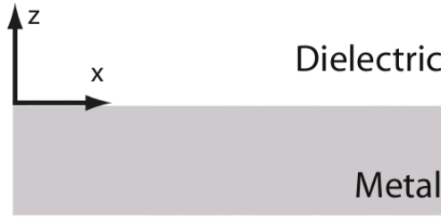
Figure 6.2: Geometry of SPP propagation at a single interface between a metal and a dielectric.
