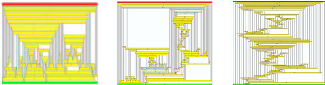
Figure 5.6: Visibility Representations of a 85-node triangulated planar graph for different st -orientations produced with PAR-STN( p ) ( p = 0, 0.5, 1 ).
