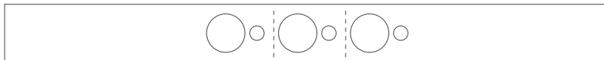
Figure 4.1: Schematic figure of the atomic structure of MnSi. The circles represent atoms and the dashed lines depict the boundaries of a unit cell. We see that this structure lacks inversion symmetry in a unit cell.[Source [7].]
