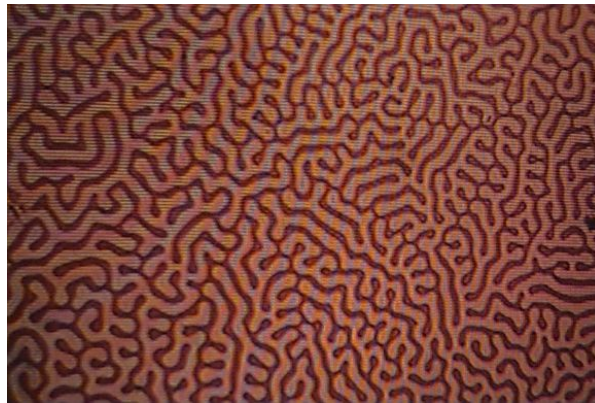
Figure 3.1: Domains in a ferromagnetic film. The magnetization points "up" in dark-coloured regions and "down" in light-coloured regions.
