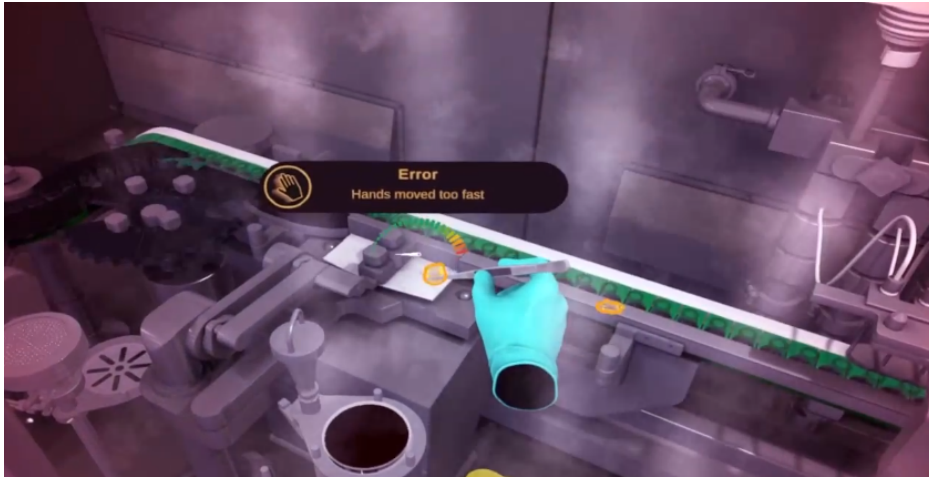
Figure 2.16: Error feedback in the Innerspace Simulator includes visual cues, such as alerts indicating when the user's hand movement is too rapid.
