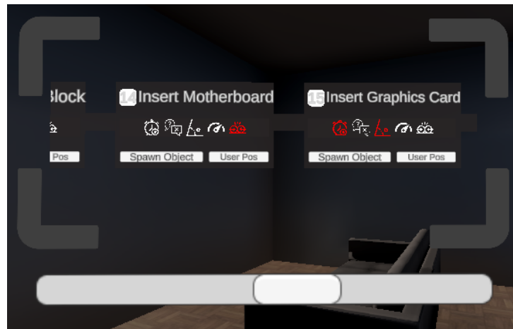
Figure 5.3: The centric part of the "World Map" UI. We can see that the collision error has been invoked in the "Insert Motherboard" action.
