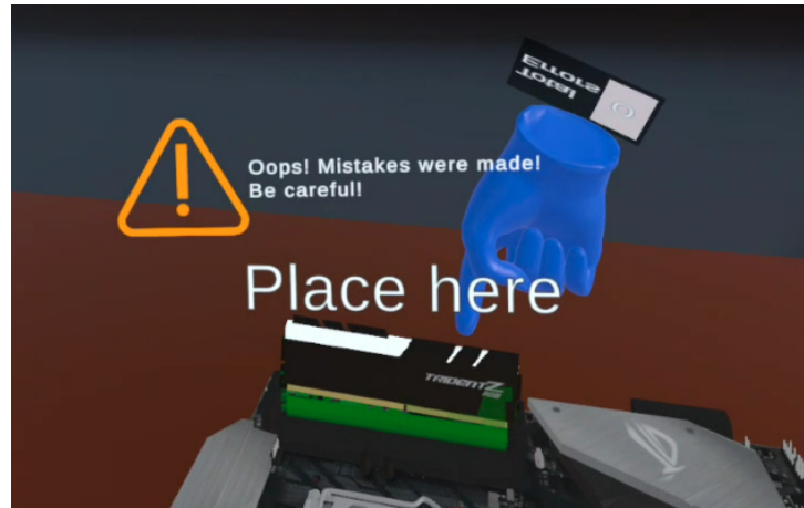
Figure 3.5: Incorrect positioning of the RAM at an improper angle results in triggering the Angle Error, prompting the system to provide visual feedback to the user.
