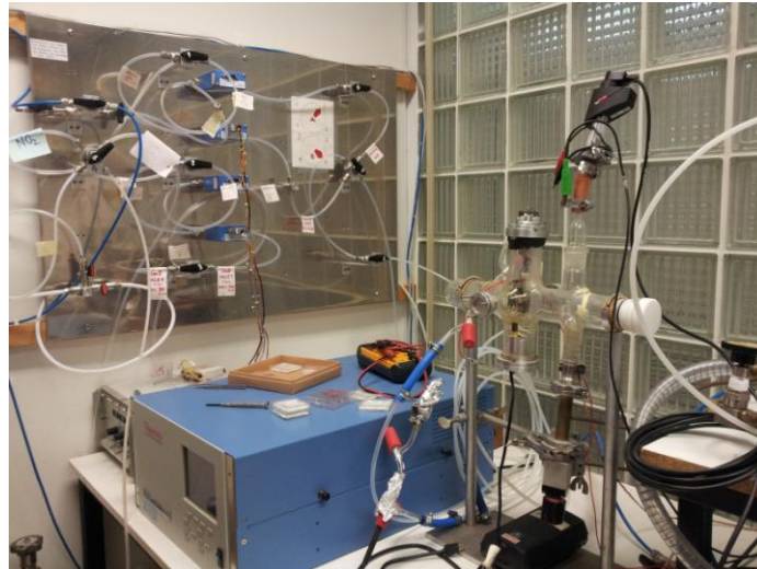
Figure 2.10: Mass flow controller system for gas sensitivity.
