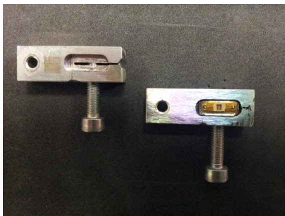
Figure 3.14: Substrate holders for SAW filters.
