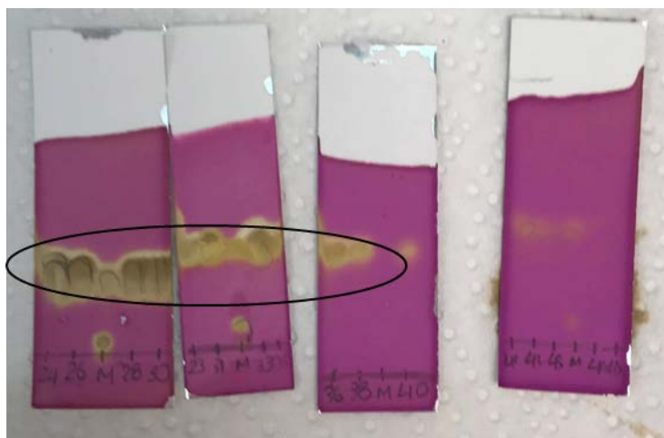
Image 2. TLC plates of the fractions eluted during the chromatographic purification of the product 3 .
