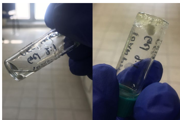
Figure 2.1: Characteristic photos of the synthesis of the PEG n (SH) 2 -TPA hydrogels: (a) before and (b) after gelation.
