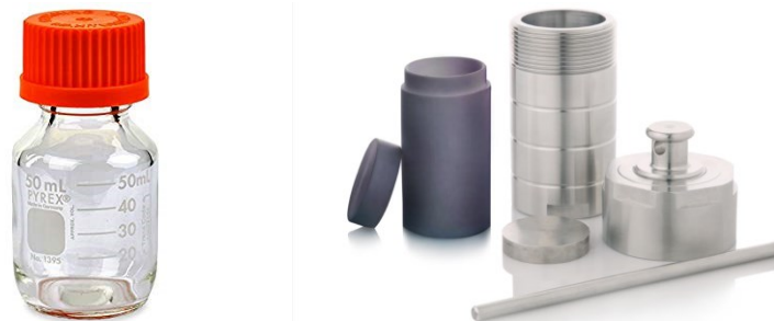
Figure 2.1 Left: Pyrex bottle with polypropylene autoclave screw cap (used at 95 °C), Right: The Teflon - lined stainless steel autoclave (used at 195 °C)
