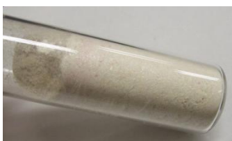
Figure 2.2.2. Light-green crystals of the SPMA monomer after purification by column chromatography and crystallization from MeOH.
