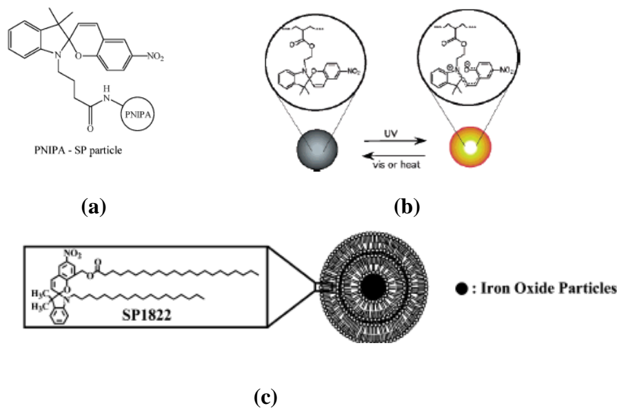
Figure 1.23. Photochromic spiropyran molecules (a) immobilized onto the surface of a polymeric sphere (b) embedded in the hydrophobic cavity of a polymeric nanoparticle (c) as part of an amphiphile forming an organic assembly for the intercalation of iron oxide nanoparticles.
