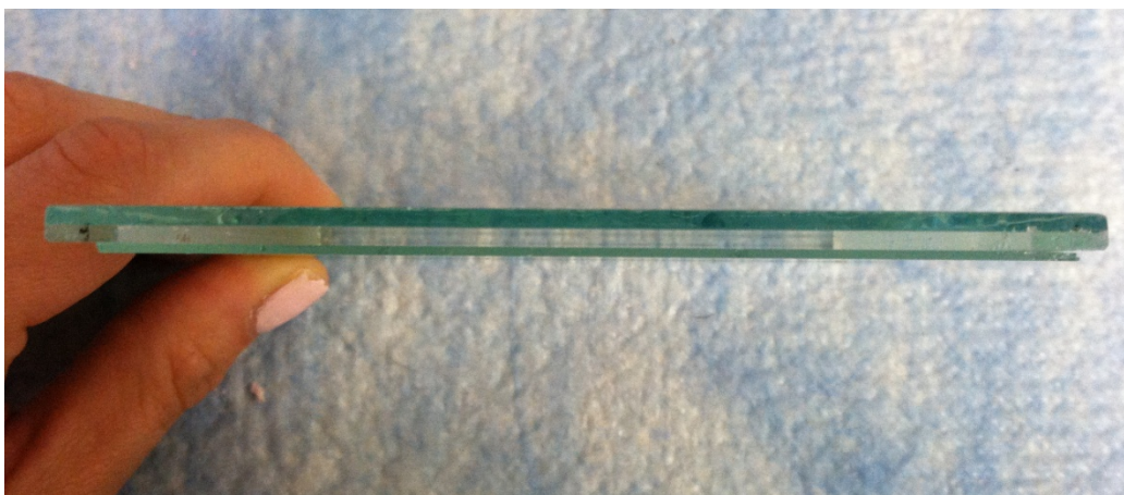
Figure 10: Proper placement of glass plates for gels.
